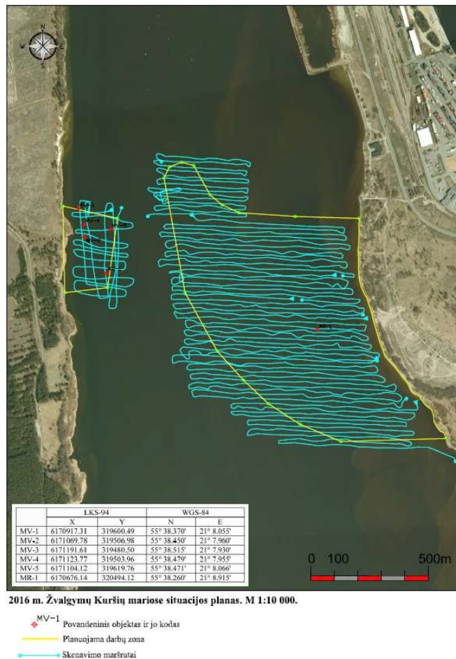
4.11.1.2 Fig. Location of underwater surveys conducted in 2016 in the planned southern gate water area of the Curonian Lagoon [19]
